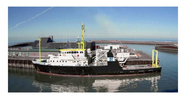
The "MULTRASHIP COMMANDER" is Multraships new, state-of-the-art oil-combat/multi-purpose/anchor-handling/towing/salvage and survey vessel for world-wide operations. The vessel can be employed in a number of roles in the offshore-, survey- and installation industry and for salvage and (oil) pollution recovery operations and rescue towages.
